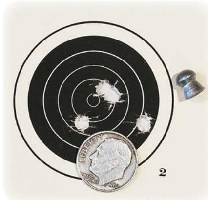
*Five JSB Exact King pellets went into 0.702 inches at 50 yards. This is the best group, but none of the six I fired was larger than 0.894 inches. This pellet is very reliable at power setting six and has proven to be the most accurate .25-caliber pellet tested in this rifle.*
