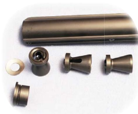
*Three high-tech baffles sit inside the frame ahead of the muzzle. They divert the compressed air after it leaves the barrel, reducing the report. A Belleville washer keeps tension on the baffles in the gun, so there's no rattling.*
