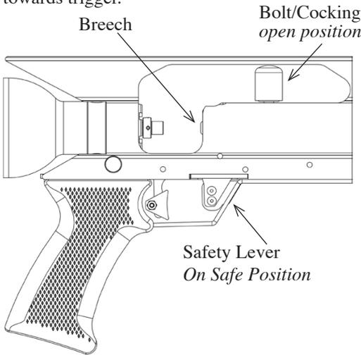
To cock the rifle, push forward on the cocking knob until the bolt is held in the open position.
