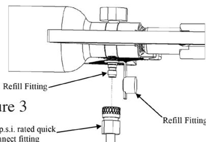
To refill your Spin-Loc Tank, attach the 3000 p.s.i. rated quick disconnect to the refill fitting. See FIGURE 3.
