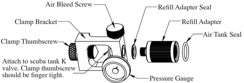
If you fill from a scuba tank that has a K-valve, the AirForce refill clamp is the way to connect your air tank. The square clamp attaches to the K-valve and mates with the O-ring in the scuba tank valve. Once the refill clamp is attached to the scuba tank, close the bleed screw and screw the air tank into the adapter.
