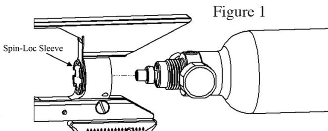
Screw the Spin-Loc Sleeve onto the air tank until it is hand tight. Make sure that the Set Screw is loose and allows the Spin-Loc Sleeve to turn freely. See FIGURE 2.
