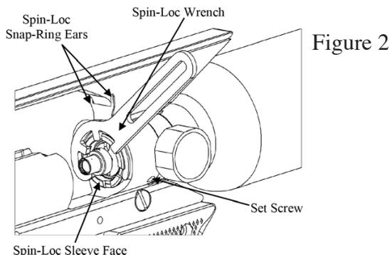
Use the Spin-Loc Wrench to tighten the air tank in place. Use CARE so you will not scratch your aluminum Frame. See FIGURE 2.
